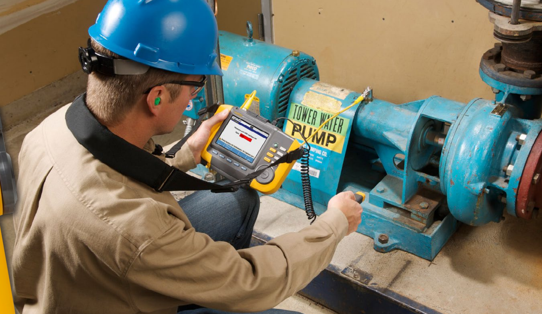
Figure 1: Understanding vibration analysis can change a run to failure system to a condition-based, proactive maintenance program
