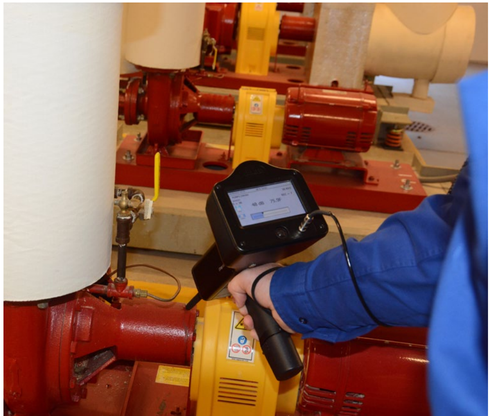
Figure 3: Today's ultrasound instrument is more than just air leaks and steam traps. This instrument is touch screen, temperature, laser, optical tachometer, camera, record audio, datalogging, Bluetooth and more. Operators with little or no experience will have a better understanding and ownership when they utilize these instruments.
