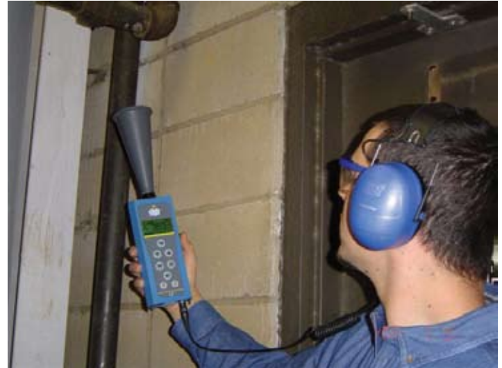
Figure 1 - A long range horn or cone is excellent for use from 5 ft. - 40 ft. (courtesy of SDT)
