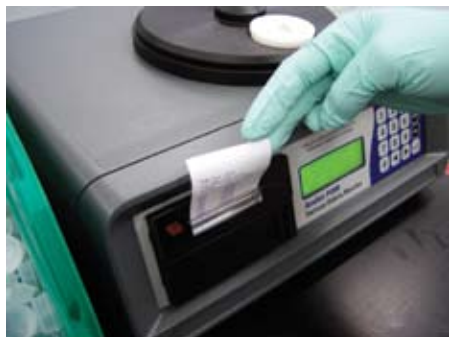
The Particle Quantifier automatically recalibrates between each sample measurement.
