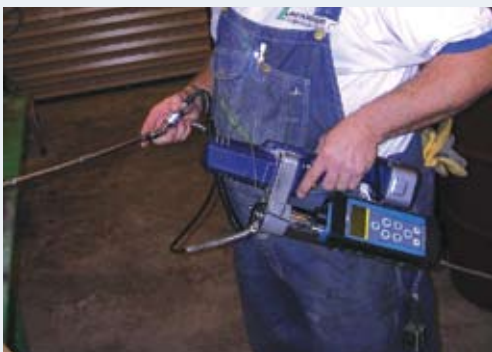
Figure 7 - Ultrasonic lubrication at Lafarge North America
