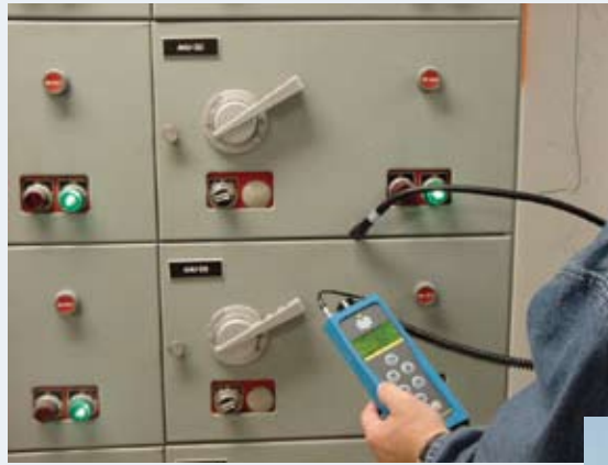
Figure 11 - Electrical inspections with ultrasound not only identify problem components but also increase safety.
